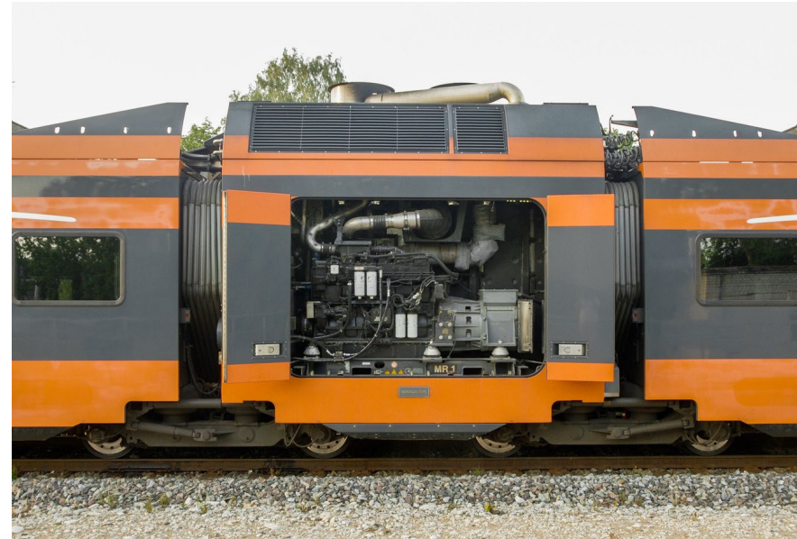
"Power Pack" car of Stadler FLIRT DMU with open bay of a diesel-generator.
